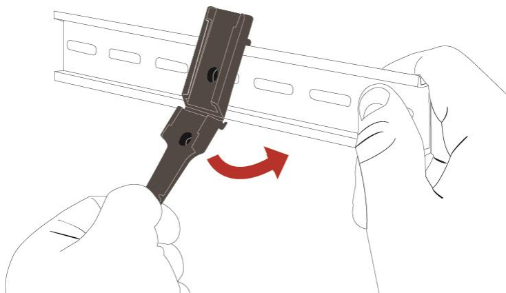
Figure 13 - Attaching the mounting bracket to the DIN rail using the V bend
