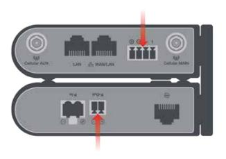
Turn on the power source. Confirm that the green power LED on both the router and switch light up when a power source is connected.
