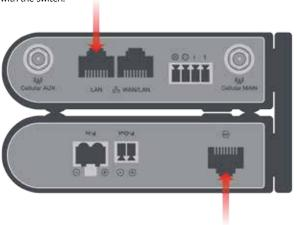
Connect network equipment to the 4 Ethernet ports on the Vodafone MachineLink Ethernet Switch. To get Gigabit speeds, ensure that you use at least Category 5e Ethernet cable.
